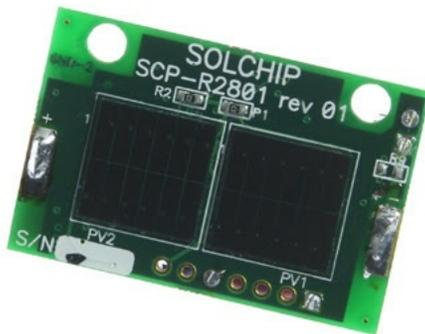
Saelig Company, Inc. has introduced the patented Sol Chip Pak™ (SCP-R2801). Their Power Modules offer day/night non-stop functionality by combining state-of-the-art solar cells, a rechargeable battery, and advanced power management circuitry. These power modules include all the components that are required to harvest energy from ambient light, charge a built-in rechargeable battery, and deliver a stable voltage to a load. [Read more...](#)
