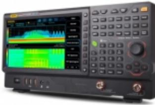
These real-time devices scan a complete frequency spectrum of 9kHz to 3.2 or 6.5GHz with a maximum sample rate of 51.2MS/s. They offer significant performance improvements over traditional swept spectrum analyzers with a 1ms full span sweep, an expanded vertical range to +30dBm, reduced phase noise to -108dBc/Hz, 1 Hz RBW (resolution bandwidth), and a reduced noise floor (DANL) to -165dBm. They can also be used in a traditional swept scan mode.
